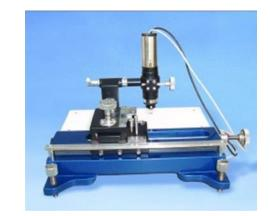
The bed is of heavy casting, thoroughly aged and machined, is fitted with leveling screws. A large platform is provided for fixing the sample.
